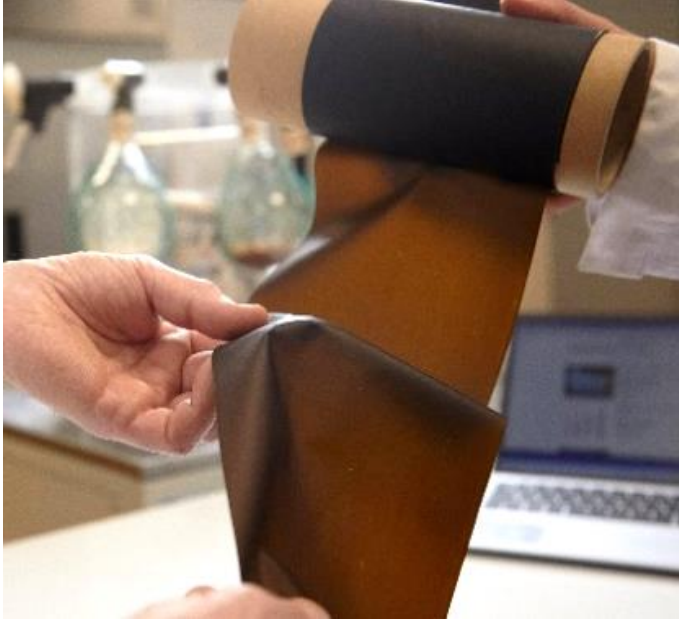
Figure 16: The seaweed-based material can be used for producers of packaging and textiles to create film and board. Photo: Oceanium
