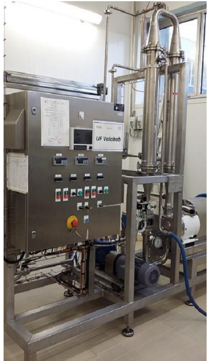
Figure 41: Ultra-filtration unit for compounds separation according to molecular weights. Image: Algaia.
