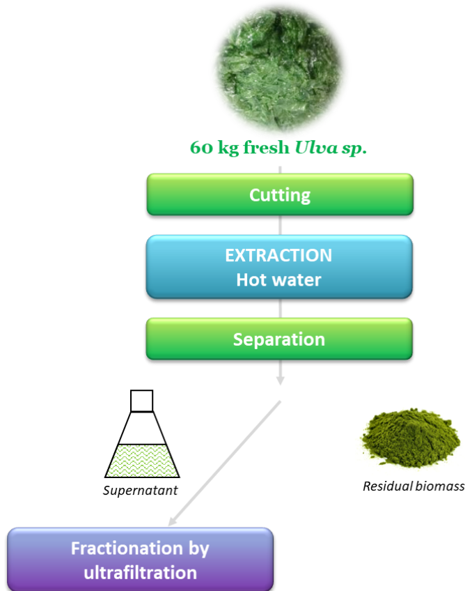
Figure 1: Diagram of the ulvan extraction protocol followed in the study.
